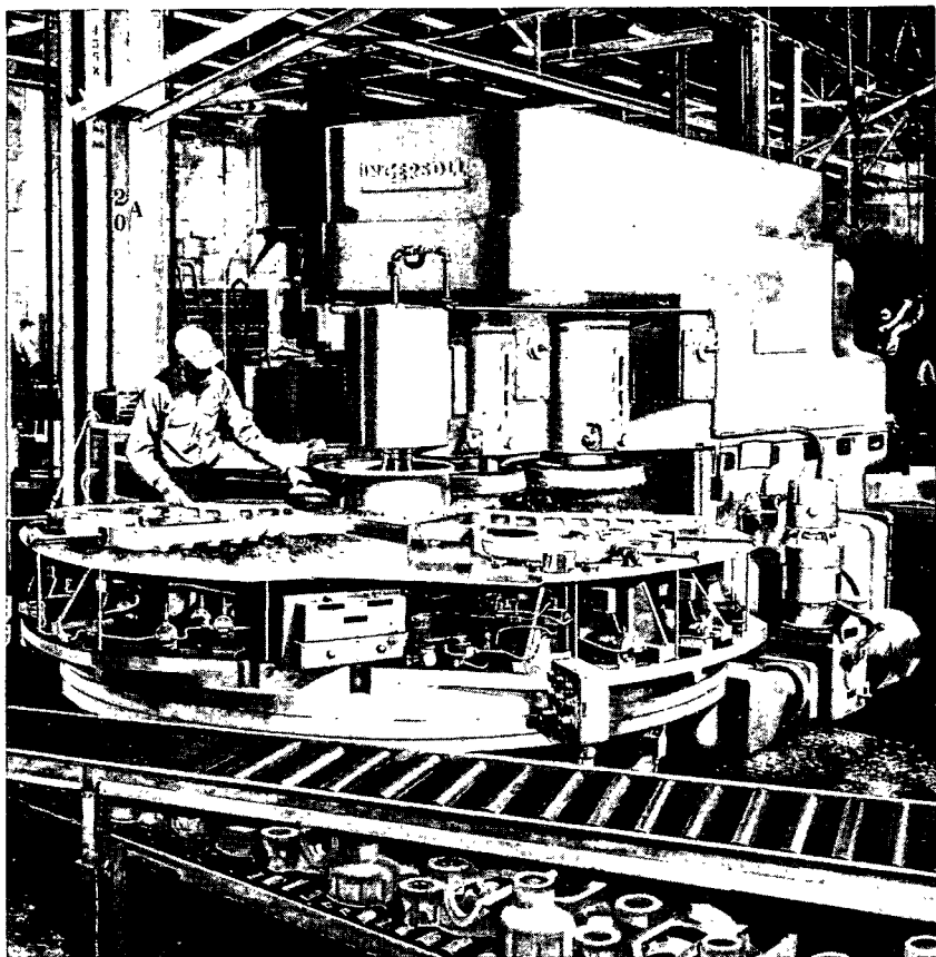
An economical answer to reducing the cost of timing gear housings for tractor engines.
