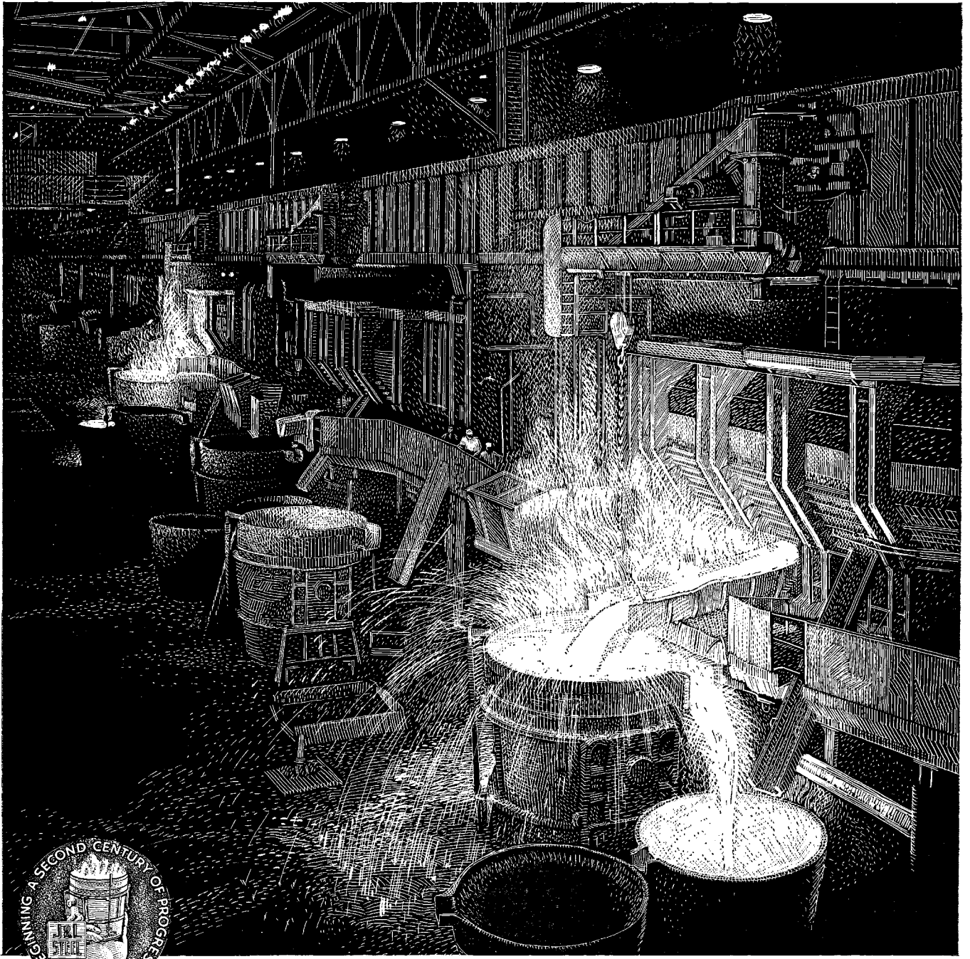
TAPPING THE NEW OPEN HEARTH'S AT J&L'S PITTSBURGH WORKS. The molten steel flowing into two giant-size ladles symbolizes J&L's capacity for modern, scientific methods of mass-producing steel.
