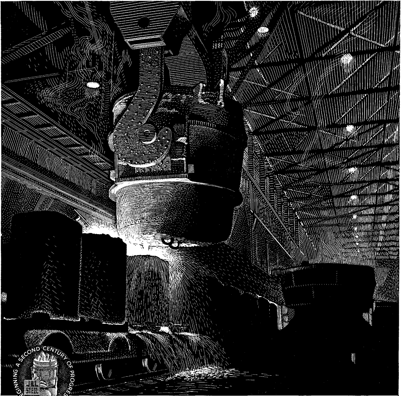
TEEMING INGOTS AT J&L. Molten steel is "teemed" into ingots after it has been "tapped" from J&L's new open hearths at Pittsburgh.
