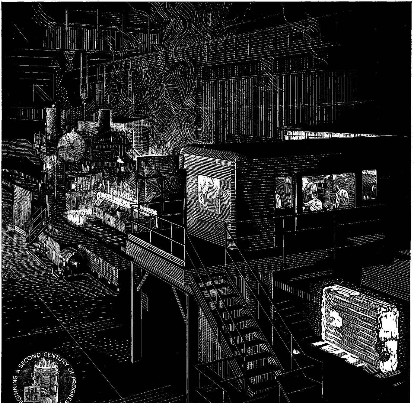
ROLLING SLABS AT J&L'S PITTSBURGH WORKS. Men in the pulpit operate controls that move the white-hot ingot to the rolls of J&L's new blooming mill. The ingot on successive passes is rolled into a slab.
