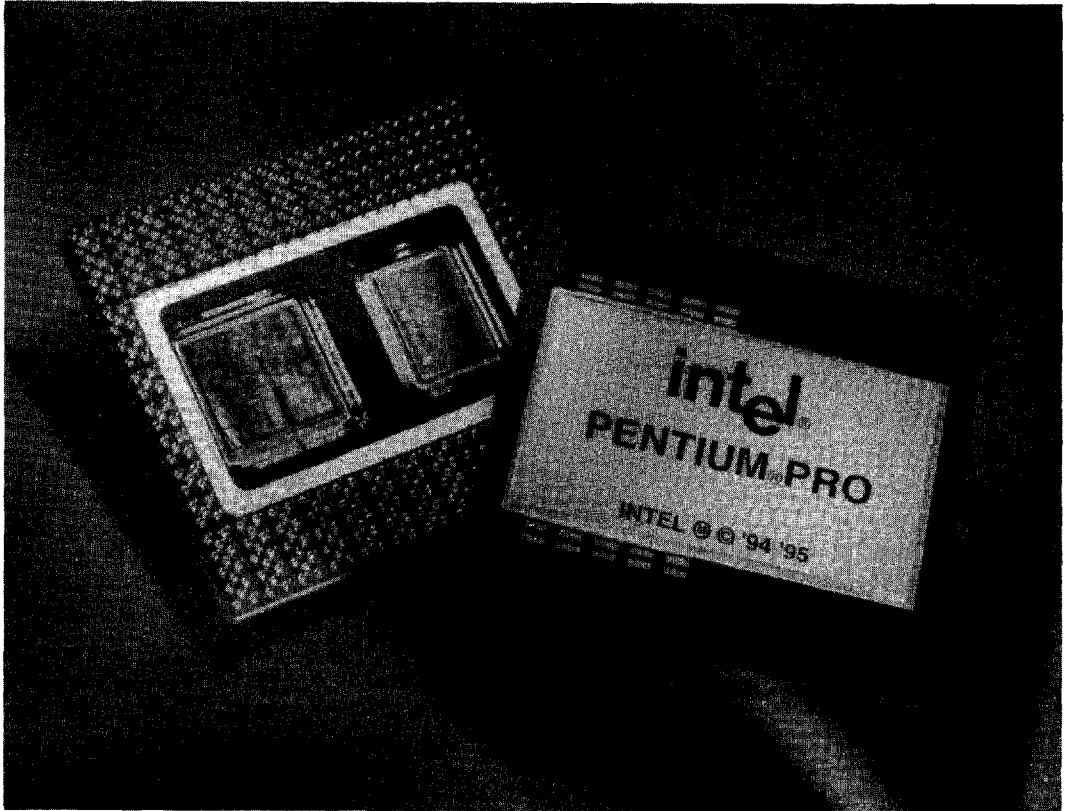
Immigrants made key contributions to the development of this thumbnail-size Pentium Pro microprocessor, which contains an incredible five million transistors. It gives personal computers the power of a high-priced office work station—for perhaps two-thirds less money.
